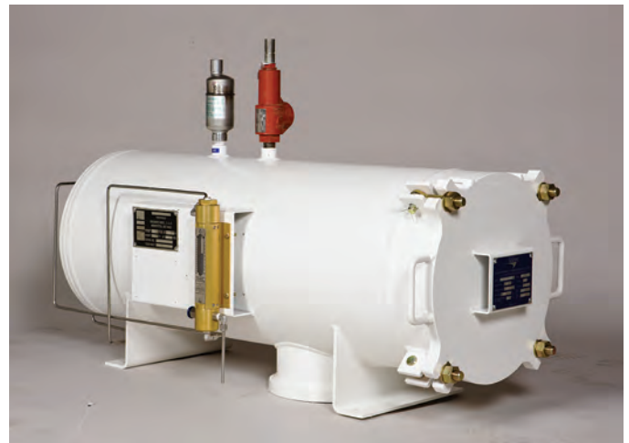
Model No. HV1633M A fully-qualified 300 USGPM Filter/Separator. End Opening unit is only 16 inches in diameter and 47 inches long.
