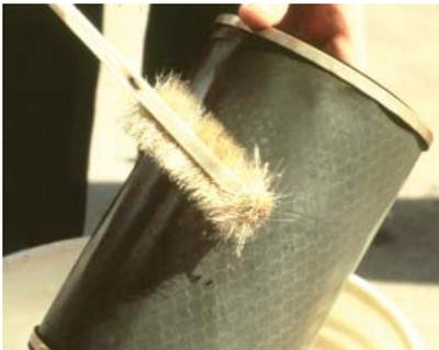
**3. SURFACE INSPECTION.** Holding the cartridge by the endcaps, visually inspect the entire surface of the screen for any nicks or cuts. If there are any visible flaws, they should be patched (see 6).
