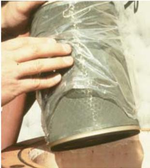
to handle the screen during removal or installation, use a clean, dry, non-abrasive material, such as a poly-bag from one of the coalescers, between your hand and the screen.
