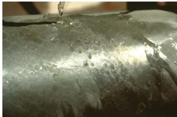
If any portion of the Teflon coated screen is wetted by the water (the water will seep into the pores of the screen; this is very obvious to the eye), the cartridge has failed the Water Test. The wetted area must be cleaned again (see 7), and the recleaned cartridge should pass the Water Test before it is reinstalled.
