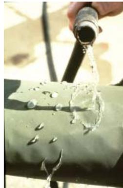
**4. WATER TEST.** Be sure that the separator is **fuel-wetted** before performing this test. Hold the cartridge by the end-cap at an angle, and gradually pour water over the entire screen surface. Do not spray the water and do not let it fall more than a distance of three inches before contacting the screen.
