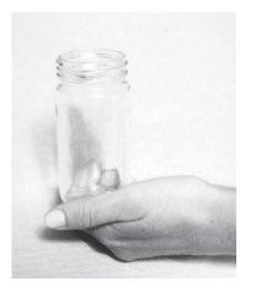
2 Take sample at receipt point; or upstream and downstream of clay vessel.
