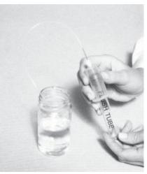
Draw the fuel sample into the SWIFTKit tube. Insure fuel level is above capillary tube.
