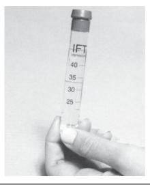
After 4 minutes, read the IFT value corresponding to the fuel/water interface level in the capillary tube.
