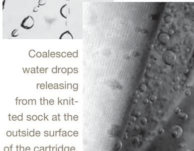
Coalesced water drops releasing from the knitted sock at the outside surface of the cartridge.
