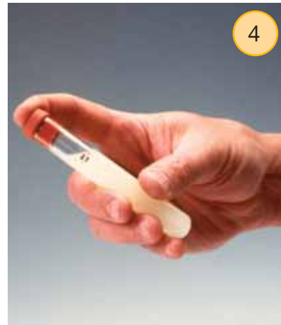
After tube fills, shake for 15 seconds. Set upright to allow powder to settle.
