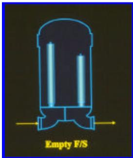
Remove air from F/S prior to introducing normal flow rate.
