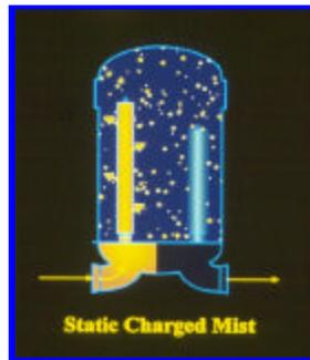
The air is not purged out. Notice the static charged mist.
