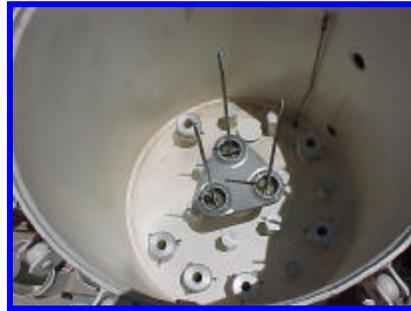
Check that the epoxy lining of the vessel is in good shape. Also, to prevent leaks, check that the lid gasket is in good shape.
