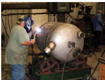
Welding a Stainless Steel Vessel
